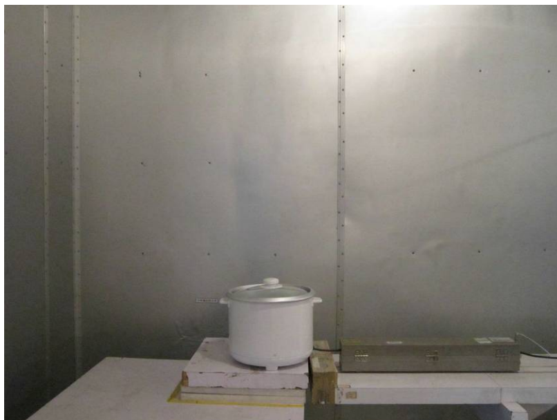
Figure B-12 Setup for disturbance power
