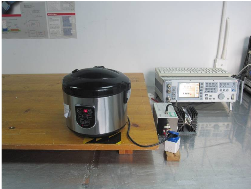
Figure B-7 Setup for Conducted Immunity
