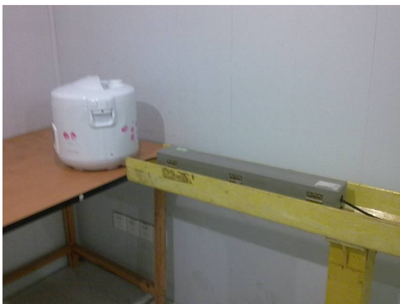
Figure B-9 Setup for disturbance power
