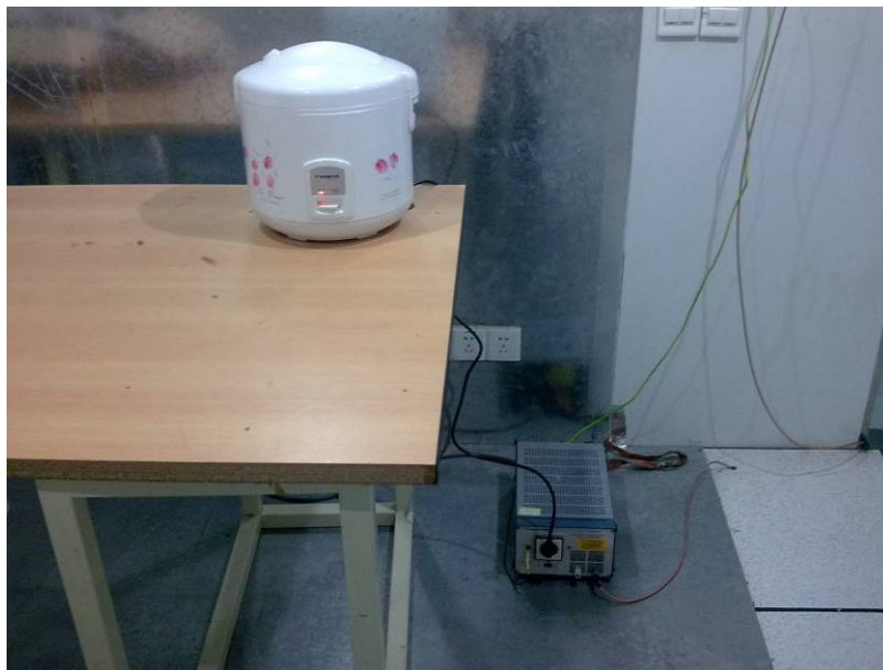
Figure B-8 Setup for conducted emission
