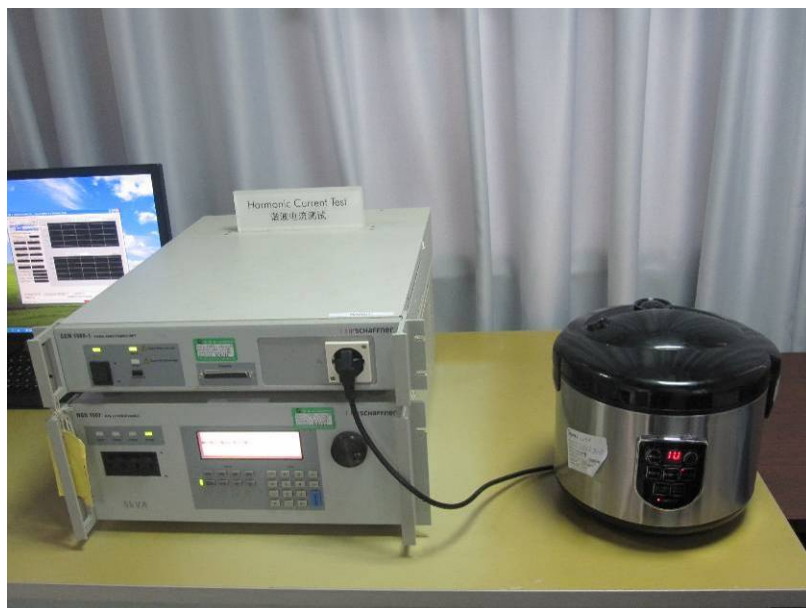
Figure B-3 Setup for disturbance power
