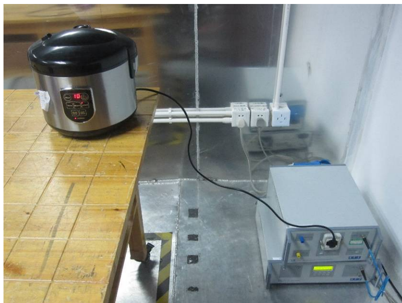
Figure B-2 Setup for discontinuous disturbance
