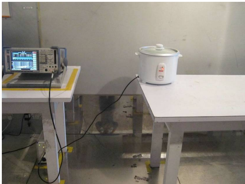
Figure B-11 Setup for conducted emission
