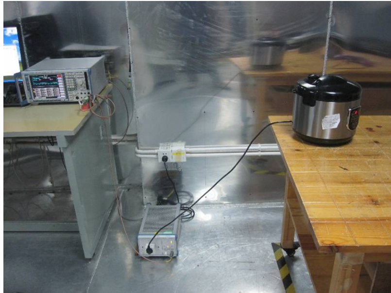
Figure B-1 Setup for conducted emission
